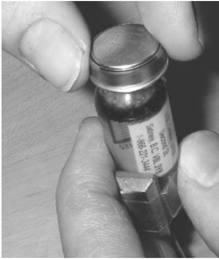
A thermal logger being affixed to a radio transmitter. The device will be waterproofed prior to deployment. Spatially-linked thermal histories can be reconstructed as per Figure 5.
