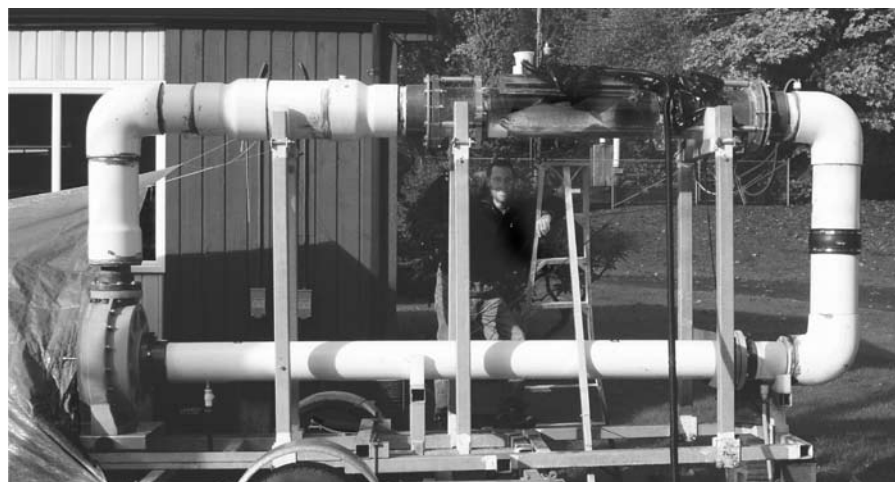
Adult sockeye salmon exposed to forced swimming in a mobile swim tunnel.
